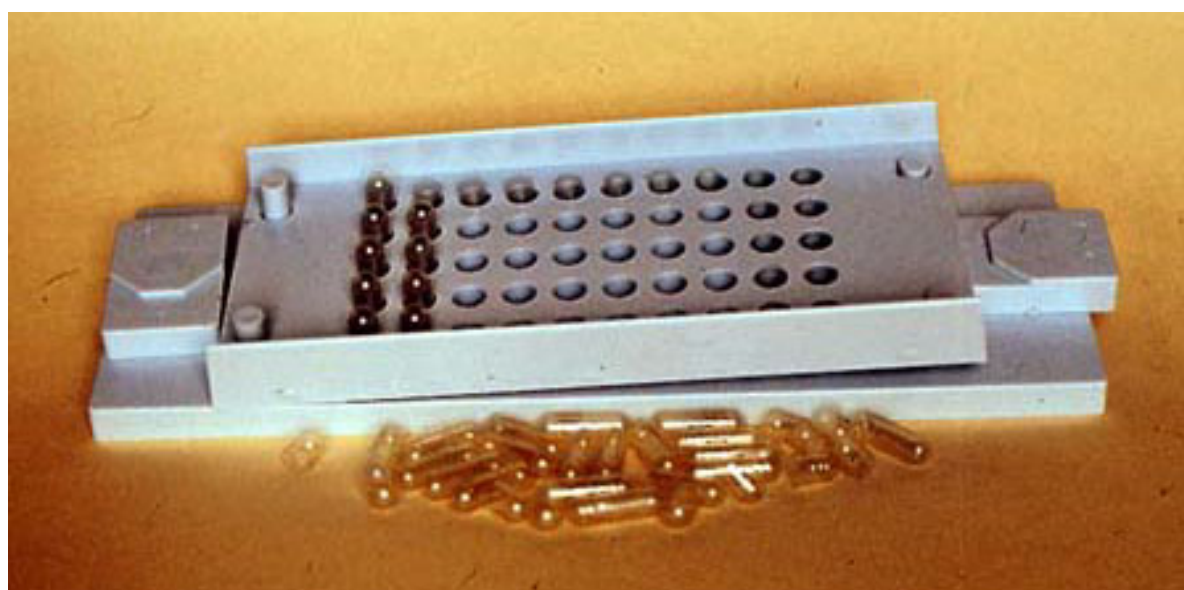
Figure 3.11: A small and cheap device for manually filling small quantities of hard gelatin capsules. With the top piece raised, as on the right, the pollen is brushed into the capsules. Once the top piece is lowered, as on the
