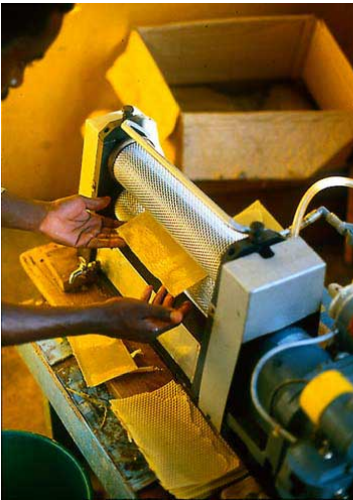
Fig 4.3 a) Melted wax starter strips from unpatterned wax sheets for topbar hives. b) Simple foundation press for single sheets requires more practice and more wax per sheet; can also be made from gypsum (plaster) using commercial foundation to prepare the plaster moulds. c) Motorised foundation rollers with moist. d) Hand-operated, low cost, plastic foundation rollers
