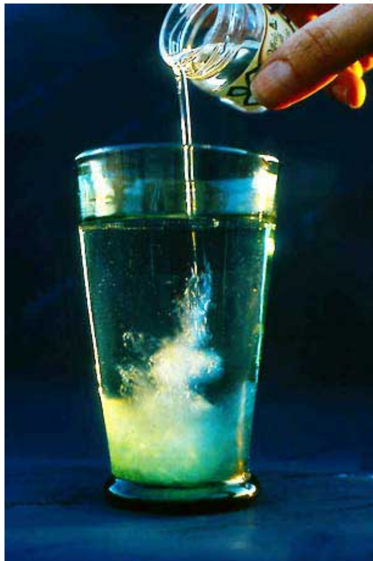
Figure 2.14 : A simple field test for adulteration of honey. a) Pure honey pours and settles without readily dissolving. b) and c) honey mixed homogeneously with equal amounts of a 70% sugar syrup (sucrose) does not pour as straight and creates turbulence and turbidity almost instantly, but particularly after pouring a greater quantity or slightly disturbing the water. The honey syrup settles irregularly at the bottom. d) 70% sugar syrup (sucrose) only; turbidity is even stronger and no distinct settlement at the bottom occurs.
