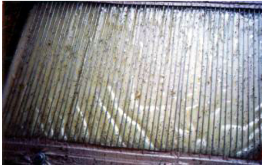
Figure 7.4 : Close-up of collecting device with stings. The steel wires are approximately 6 mm apart and suspended 1 to 3 mm above the thin silicon rubber film or directly above the glass plate in other models. The wires are alternately grounded and charged to a maximum of 33 volts. A lower voltage is effective, too. Preferably a collecting surface should be used which does not make bees loose their sting. (Courtesy of B. Weeks)
