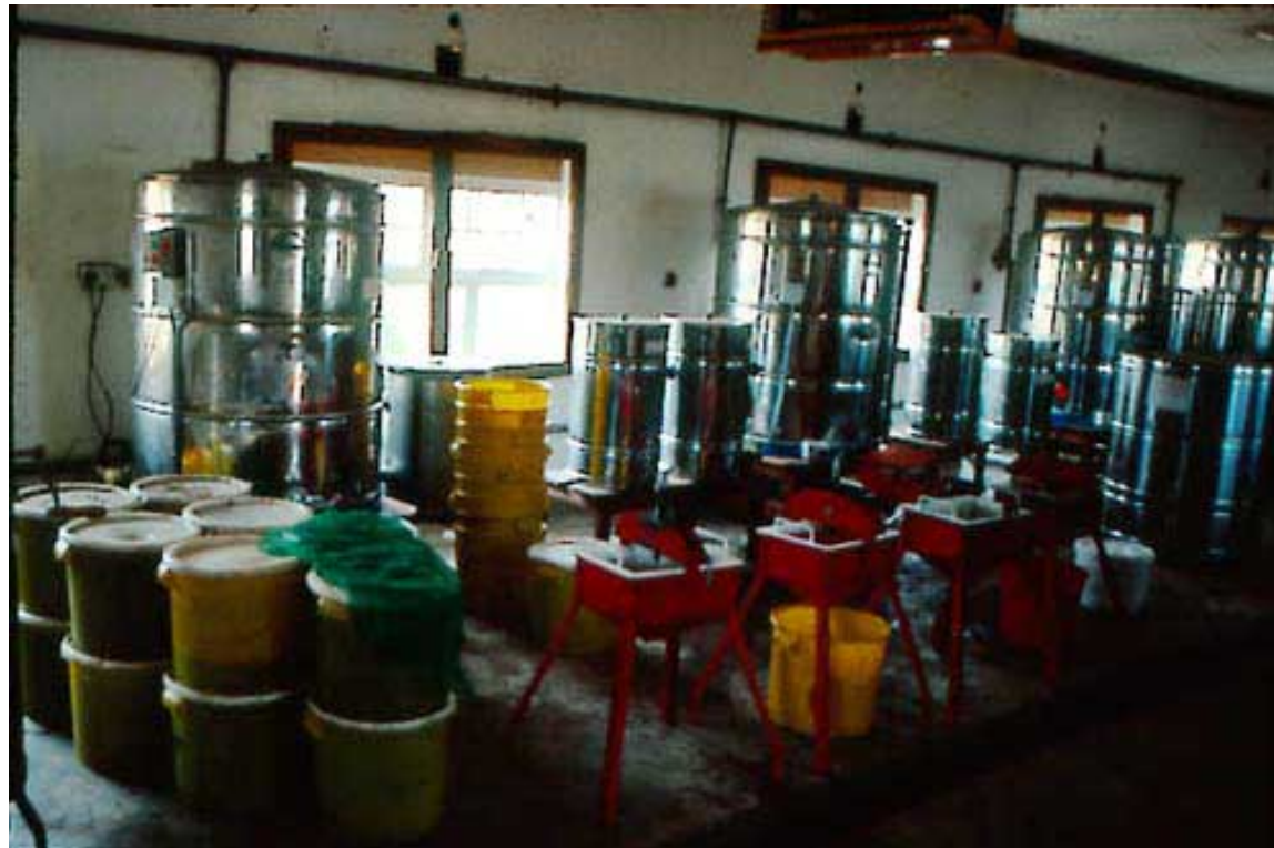
Figure 2.6 : Honey presses in the foreground and water jacketed settling tanks in the background at the honey processing centre of Northwestern Bee Products, Kabompo, Zambia, which buys, processes and exports honey and wax from mostly traditional barkhive beekeeping.
