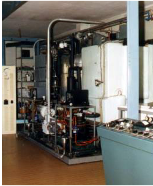
Figure 6.9: Industrial size freeze-drier in room with controlled environment (Courtesy of Ghimas SpA).
