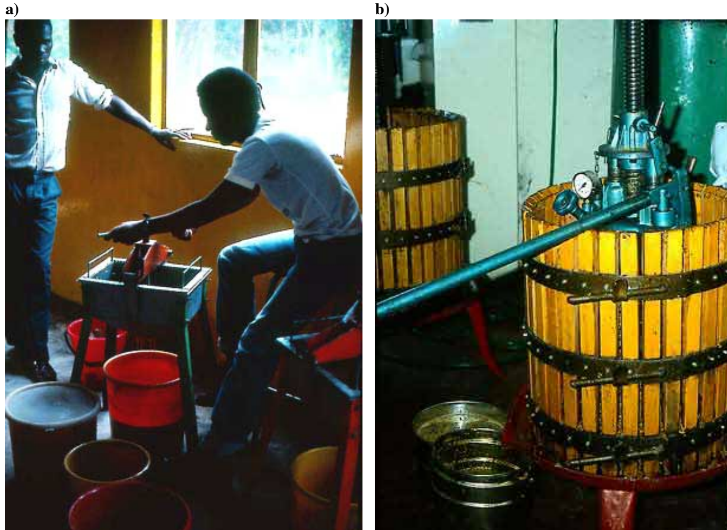
Figure 2.9: a) Small, common honey press in Zambia; b) Larger honey press used to squeeze honey from cappings in Italy.
