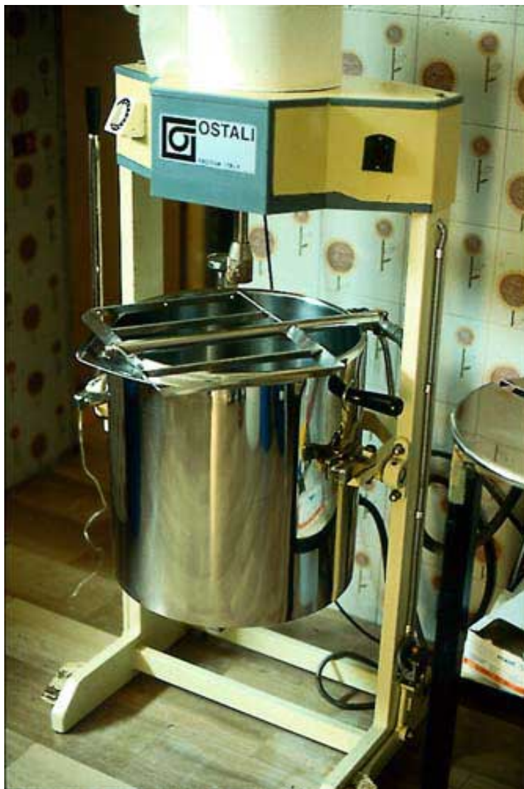
Figure 9.7: A simple, small to medium size paddle mixer with water jacketed bowl for temperature control of the mix. During operation, the paddles are equipped with plastic scrapers which allow very close contact between paddle and vessel, thus avoiding any "dead" spaces.
